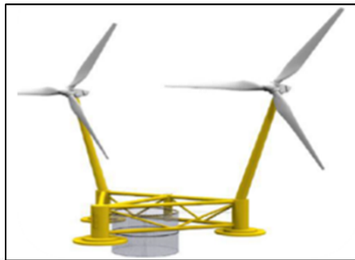
Fig 1 - Schematic view of the joint unit W2Power prototype
